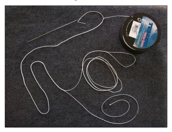
The needle is now reinserted into the new line about half an inch away from the spot where it entered the old line. The tag end of the old line now goes into the wire loop (or latch), and it will be threaded inside the new line for about three feet.
